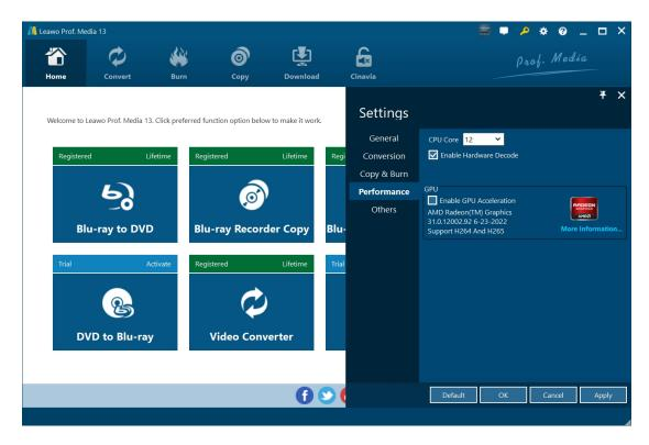
On "Performance" tab, set CPU core, choose to enable hardware decode, and choose GPU acceleration.
